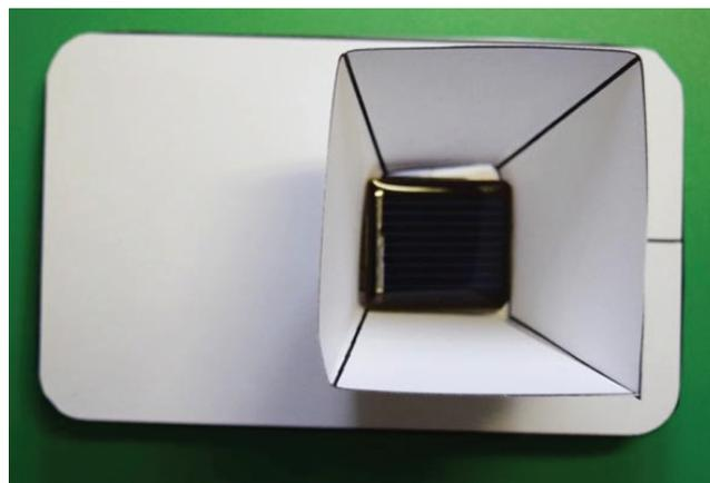
**Figure 5.2:** Example of a mini solar car with vertical reflector attached. (UMaine Extension 4-H Photo, Sarah Sparks)
