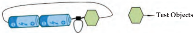
Figure 1.4: Here is how you need to set up the circuit to test conductivity (tape the batteries together to keep them from separating) (UMaine Extension 4-H Graphic, D.O. Neill)
