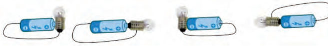
Figure 1.2: Here are some of the different orientations of the circuit with the 1.5V bulb. (UMaine Extension 4-H Graphic, D.O. Neill)
