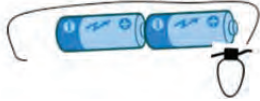
Figure 1.3: Here is how you need to set up the circuit for the LED light (tape the batteries together to keep them from separating) (UMaine Extension 4-H Graphic, D.O. Neill)
