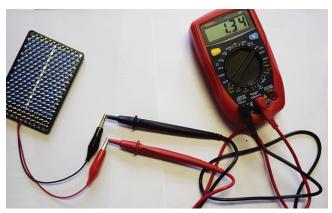
**Figure 2.5:** Sample set up of solar panel with multi-meter. (UMaine Extension 4-H Photo, Sarah Sparks)
