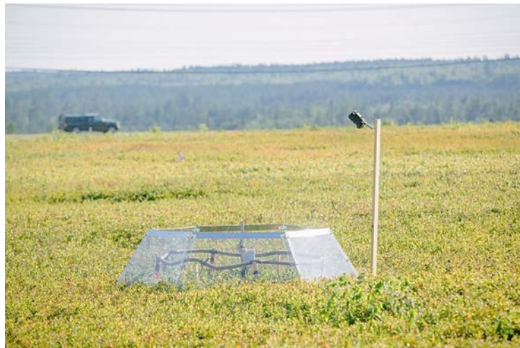
Figure 1. Climate change chambers used to study warming effects on wild blueberries and pests. Chambers are installed at Blueberry Hill Research Farm, Jonesboro, ME.
