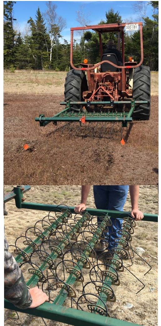
Figure 1. Williams flex-tine weeder at Blueberry Hill Farm, May 2019.
