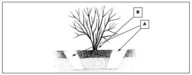
planted too deeply, or if they are placed on backfill that later settles and effectively "plants them" too deeply, then they are subject to two serious problems. First, roots require oxygen to function, and the oxygen level several inches below the surface is low. If roots cannot access oxygen, then they cannot grow, and the plant will decline and possibly die.
