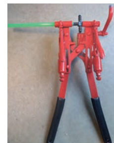
Two-handed tubing tool for grasping tubing, pulling it tight, and securing fittings.
