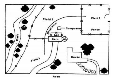
Example of a property map showing how to manage horses and their waste. Runoff should not be allowed to discharge directly into a stream or other water body. Placing a diversion above a high-use area may prevent outside runoff from flowing across the barn or manure containing paddock and storage areas. A diversion placed below the high-use area will help direct runoff from the lot away from water or wet areas.4
