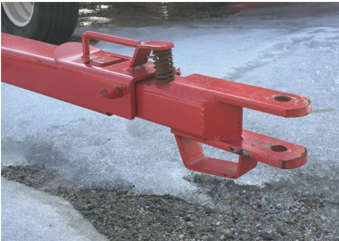
Telescoping tongue in the retracted (locked) position
