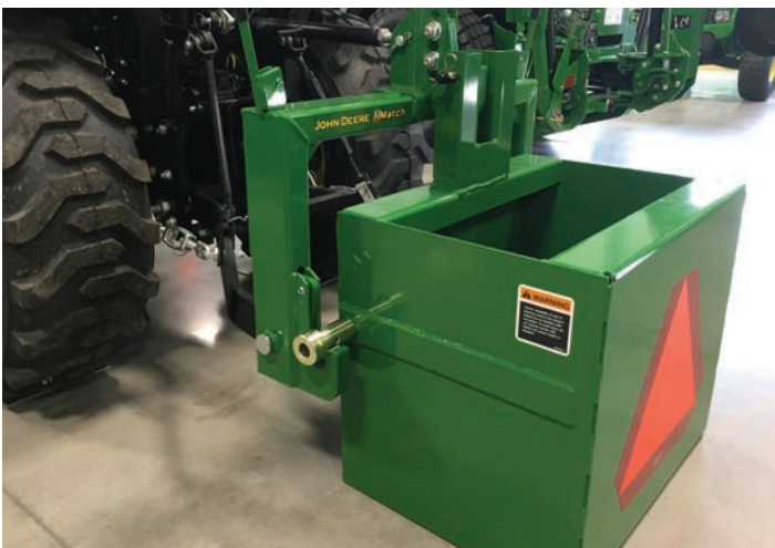
Typical quick connector system
