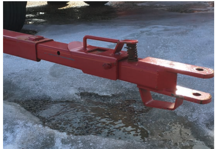
Extended telescoping tongue for easy connecting
