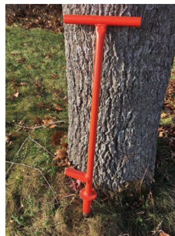
Upright tree dibbling tools allow for creating holes relatively easily for transplanting through heavy cover crop residue. Photo: Natalie Lounsbury.
