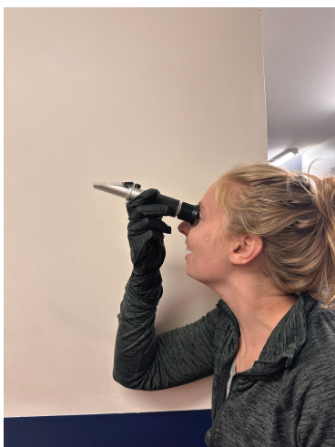
Figure 2. Using a refractometer.
