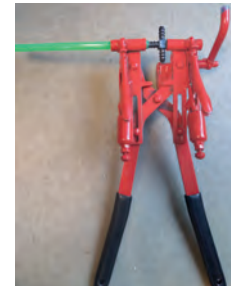
Two-handed tubing tool for grasping tubing, pulling it tight, and securing fittings.
