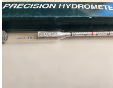
A maple syrup hydrometer is used to measure sugar concentration by the level that it floats.
