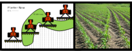
Figure 1: Use of GPS to protect inputs from overlapping. Photo Courtesy: Solberg et al., 2006
